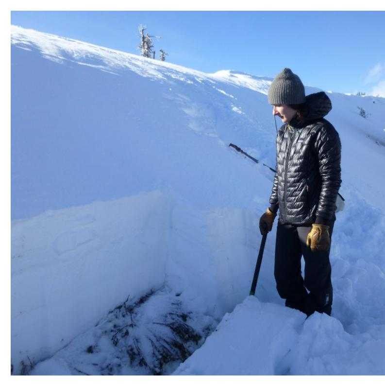
This stability test broke and propagated (ECTP17) on a 5cm layer of moist facets at the ground. These facets have not been causing widespread problems, but should not be ruled out. Photo: GNFAC
