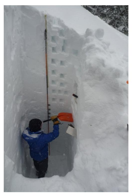
A snow ranger from Cooke City and a member of the USGS completed the daunting task of trying to find the ground under more than 10' of snow. This pit was dug near Daisy Pass and had a depth of 133 inches. The main instabilities in the snowpack exist in the top 1-3' and mostly involve wind blown snow. Photo: M. Dixon
