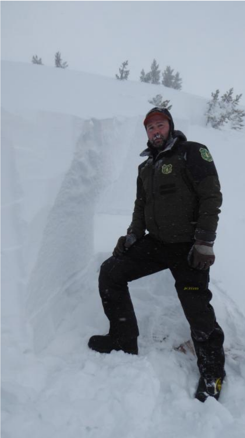
Ian Hoyer stands next to the crown where we dug a snowpit and investigated the snow structure. The crown averaged 4-5 feet deep. Near his right knee is the layer of weak faceted snow that broke 40 cm above the ground. Above this layer was a thick slab of windblown snow. Photo: GNFAC
