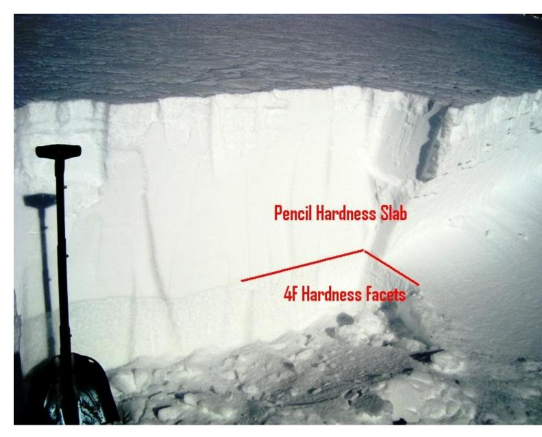
This snowpit was dug in the crown of the slide that a snowmobiler triggered Dec 27. A layer of weak facets could not support the hard slab of wind blown snow plus the rider. The steepest part of the slope was 37 degrees.
