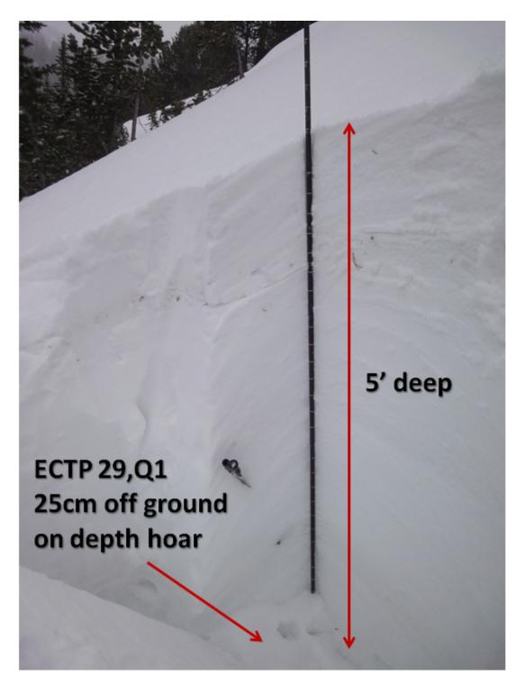
This pit was dug on a north facing slope at Lionhead. The ECT failed on 29 taps on large depth hoar crystas less than a foot off the ground. Although it would be difficult to trigger when it is this far under the surface, in areas wher the snowpack is thinner a snowmobiler could initiate a fracture that would propagate to deeper slopes like this one. Photo: GNFAC
