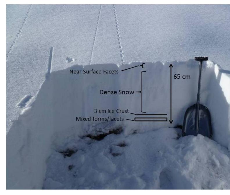
The snowpack near Bridger Bowl is roughly 2 ft deep on the upper mountain. The pack consists mainly of dense, well bonded snow; however, an ice crust in the lower pack rests on a weaker layer of mixed forms and facets. This layer did propagate during an ECT indicating it has the ability to propagate a fracture. Currently, there is not enough snow to make this layer a major problem, but with a heavy load it could become reactive.
